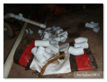
PVC joints used to make mock bridge.
