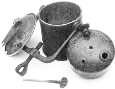
Figure 1: Pinnacle Major Carbide Hand Lamp disassembled. S. McCabe Collection. Photo: Ken Keane
