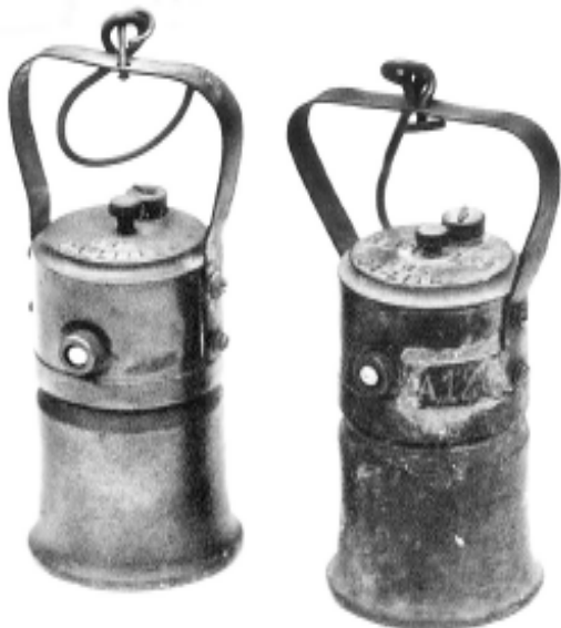
Figure 18: DA-Lite (plain) and DA-Lite NBH Ltd: Carbide Hand Lamp. S. McCabe Collection. Photo: Ken Keane
