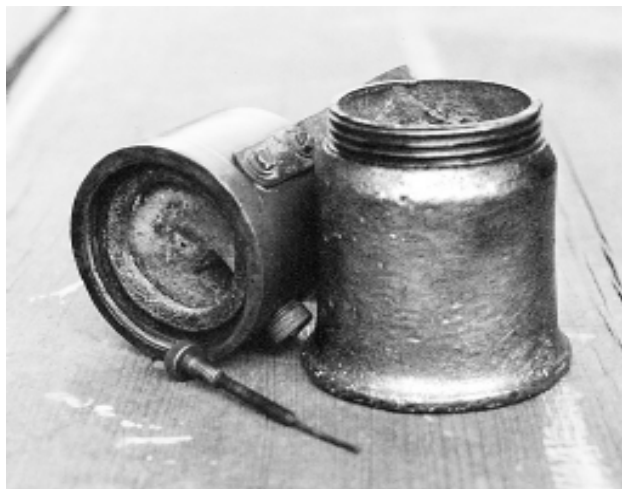
Figure 17: DA-Lite (complete) and disassembled carbide hand lamps. S. McCabe Collection. Photo: Ken Keane.
