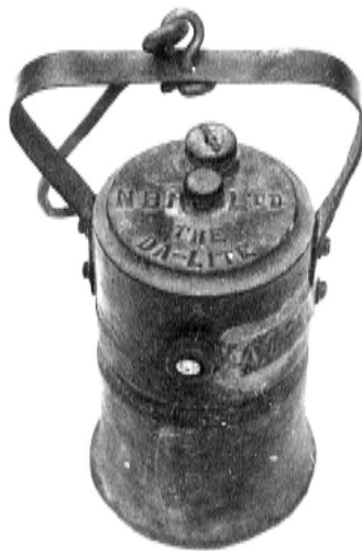
Figure 16: DA-Lite NBH Ltd. Carbide Hand Lamp S. McCabe Collection Photo: Ken Keane
